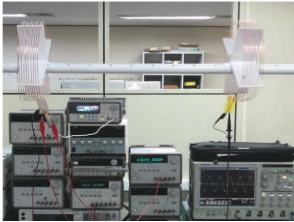
Figure 6 Photograph of the experimental setup of WPTS. [Color figure can be viewed in the online issue, which is available at wileyonlinelibrary.com ]
